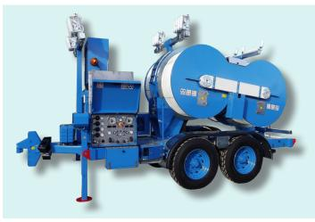
Hydraulic tensioner fit to string 1, 2, 3 or 4 conductors. Two hydraulic circuits allow to tension at constant force even varying the speed of stringing. The two circuits can be used independently or simultaneously, with automatic forces partition. Equipped with engine for pull-back performances. In pull-back mode, two hydraulic circuit allow to vary the speed in both directions, allowing to use one of the hydraulic circuits or both them matched.
