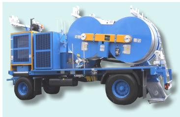
Hydraulic machine designed to operate both as a tensioner and as puller, fit to string 1, 2, 3 or 4 ropes or conductors. Two hydraulic circuits allow to tension at constant force even varying the speed of stringing. The two circuits can be used independently or simultaneously, with automatic forces partition. In puller mode, 2 closed hydraulic circuits allow to vary the speed in both directions, allowing to use one of the hydraulic circuits or both of them matched.
