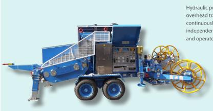
Hydraulic puller fit to pull one or two ropes in stringing operations of overhead transmission lines. Two hydraulic circuits allow to continuously vary the speed in both directions by operating two independent control devices. The two circuits may also be matched and operated together by one control device.
