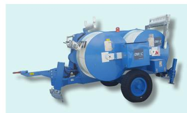
Hydraulic tensioner fit to string 1, 2, 3 or 4 (up to 6 on demand) conductors. One hydraulic circuit allows to tension at constant force even varying the speed of stringing. Equipped with engine for pull-back performances.
