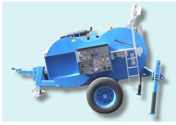
Hydraulic machine designed to operate both as a tensioner and as puller, fit to string one or two ropes or conductors. Two hydraulic circuits allow to tension at constant force even varying the speed of stringing. The two circuits can be used independently or simultaneously, with automatic forces partition. In puller mode, 2 closed hydraulic circuits allow to vary the speed in both directions, allowing to use one of the hydraulic circuits or both of them matched.
