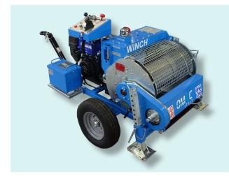
Hydraulic winch fit to pull one rope in service operations such as setting-ups and adjustment of transmission lines and underground cables laying.
