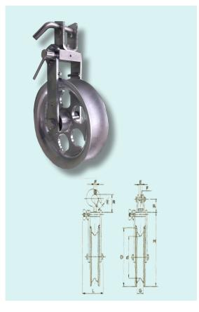
Running out block fit for stringing shield wires. Galvanized steel sheave mounted on ball bearings. Galvanized steel frame with non-fleeting device.
