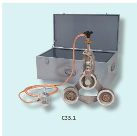
Grounding device to be used while stringing overhead conductors or pulling ropes. Aluminium alloy sheaves with bushes grant a good sliding and electric continuity even on junction points. Contrast spring for a safe and continuous contact on conductors with junction clamp. Supplied with:
