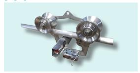
Device for measuring the length of ropes and cables. Measuring wheel made of steel. Idle wheels made of aluminum or nylon. Fit for ropes with diameter up to 50 mm.
