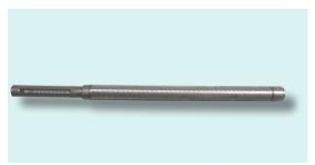
Thermometer for conductors, made up of a bulb shaped and dimensioned like a conductor. Column reading, scale in Celsius degrees (°C).
