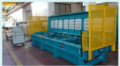
Traction bench designed to test and verify the resistance to traction (breaking force) of any part or group.
