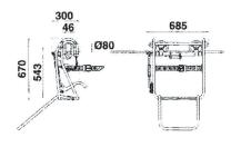
Line car for single-conductor lines. Fit for 1 or 2 linemen. Aluminium alloy structure with nylon wheels mounted on ball-bearings. Parking brake. Equipped with metercounter.
