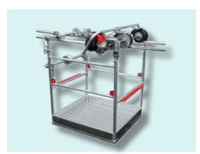
Motorized line-car for twin conductor lines (2 cond.). Made of light alloy structure with wulcolan wheels mounted on ball-bearings. Transmission axle with high grip rubber wheels. Stationary brake and metercounter.
