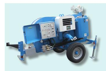
Hydraulic tensioner fit to tension one conductor or fiber optic cable.
