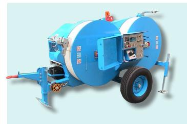
Hydraulic tensioner fit to string one conductor or fiber optic cable. One hydraulic circuit allows to tension at constant force even varying the speed of stringing. Equipped with engine for pull-back performances.
