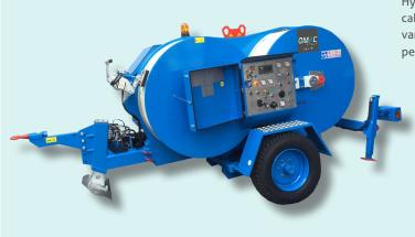
Hydraulic tensioner fit to string one or two conductors or optical fiber cables. One hydraulic circuit allows to tension at constant force even varying the speed of stringing. Equipped with engine for pull-back performances.
