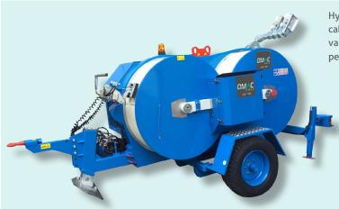
Hydraulic tensioner fit to string one or two conductors or optical fiber cables. One hydraulic circuit allows to tension at constant force even varying the speed of stringing. Equipped with engine for pull-back performances.
