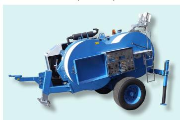
Hydraulic tensioner fit to string one or two conductors. Two hydraulic circuits allow to tension at constant force even varying the speed of stringing. The two circuits can be used independently or simultaneously, with automatic forces partition. Equipped with engine for pull-back performances. In pull-back mode, two hydraulic circuit allow to continuously vary the speed in both directions, allowing to use one of the hydraulic circuits or both of them matched.
