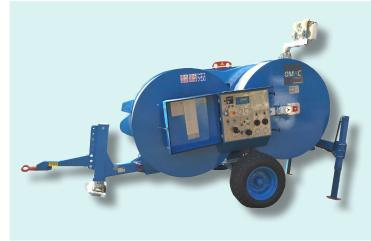
Hydraulic machine designed to operate both as a tensioner and as puller, fit to string one rope or conductor. One hydraulic circuit allows to tension at constant force even varying the speed of stringing. In puller mode, one hydraulic circuit allows to continuously vary the speed in both directions.
