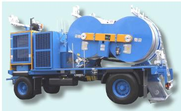
Hydraulic machine designed to operate both as a tensioner and as puller, fit to string 1, 2, 3 or 4 ropes or conductors.
