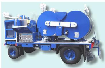
Hydraulic machine designed to operate both as a tensioner and as puller, fit to string 1, 2, 3 or 4 ropes or conductors.
