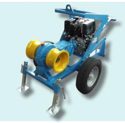
Mechanical winch fit to pull one rope while laying underground cables. The motion to the capstans is transmitted through a multiple-disk clutch and a gearbox, operated by means of 2 levers.
