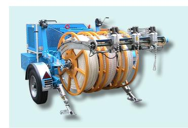
Trailer designed for transporting reels as well as for recovering and releasing ropes and conductors to/from wooden or steel reels. The trailer can host up to 3 or 4 reels. The reels, operated by a hydraulic motor, allow to recover the wires (like a puller) and to release them (braked tension).
