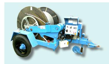
Trailer for reels, fit for recovering and releasing ropes and conductors to/from wooden or steel reels. The reel, operated by a hydraulic motor, allows to recover the wire or conductor (puller use) and to release it (tensioner use).
