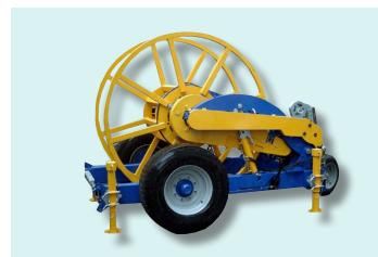
Reel-winder trolley designed for recovering/pulling and releasing ropes and conductors to/from steel reels. The reel is operated by a hydraulic motor fed by a separate power unit or by the auxiliary hydraulic circuit of a puller, tensioner or puller/tensioner.
