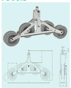
Rollers for stringing single conductor made of galvanized steel frame with openable side. N° 4 nylon sheaves mounted on sealed ball bearings.
