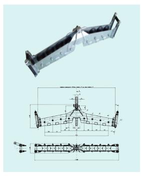
Rollers/pulley designed for stringing conductors up to diameter 60 mm. Made of electrowelded and galvanized steel. Nylon rollers turning on bearings. Flexible fittings.
