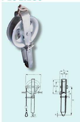
Counter-pull running-out block. Galvanised steel frame, openable side, with swivelling hooks on the ends. Automatic releasing device for recovering the unit. vers. AS Galvanised steel pulley mounted on ball bearings.
