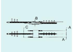
F153.2...F Fixed type running board for 2-bundle conductor, fit for connecting the pulling rope to 2 conductors. The running board is made up of:
