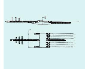
**Fixed type** running board for 6-bundle conductors fit for connecting the pulling rope to 6 conductors. The running board is made up of:
