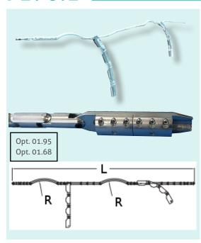
Antitwisting counterweight fit for stringing overhead fiber optic cables (OPGW). The counterweight allows to prevent the cable from twisting during the passage in the running out blocks. Its shape is designed for passing in the grooves of the running out blocks without damaging the cable. To be matched with a pulling stocking (not supplied - to be quoted on request).
