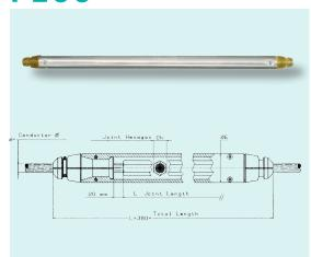
Joint protector made up of two galvanised steel shells. The ends are shaped to host the rubber protections. It is fit to limit the bending radius of the conductor during the passage in the running out blocks.
