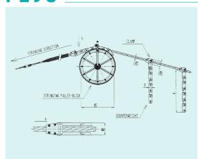
Antitwisting counterweight fit for stringing overhead fiber optic cables (OPGW). The counterweight allows to avoid the cable twisting during the passage in the running out blocks. Its shape is designed for passing in the grooves of the running out blocks without damaging the cable. A pair of nylon liners prevents damages to the cable. Supplied in metallic case.
