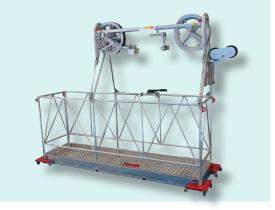
Line car for single-conductor electric lines. Fit for 2 linemen. Aluminium alloy structure with nylon wheels mounted on ball-bearings. Parking brake. Equipped with metercounter.
