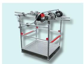
Motorized line-car for twin conductor lines (2 cond.). Made of light alloy structure with wulcolan wheels mounted on ball-bearings. Transmission axle with high grip rubber wheels. Stationary brake and metercounter.
