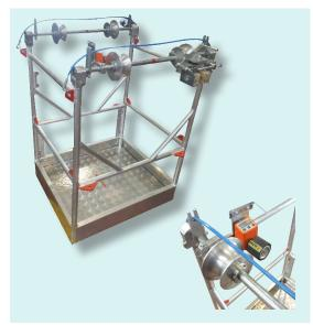
Line-car for twin conductor lines (2 cond.). Made of light alloy structure with nylon wheels mounted on ball-bearings. Stationary brake and metercounter.
