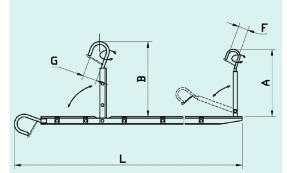
Suspension ladder fit for vertical and horizontal use.
