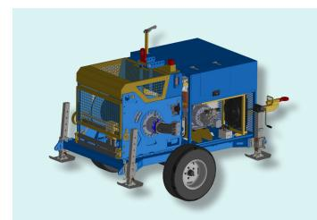
Hydraulic winch fit to pull one rope in service operations such as setting-ups and adjustment of transmission lines and underground cables laying. Direct pull on the drum. One closed hydraulic circuit allows to continuously vary the speed in both directions by operating one control device.
