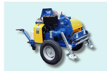
Hydraulic winch fit to pull one rope in service operations such as setting-ups and adjustment of transmission lines and underground cables laving.
