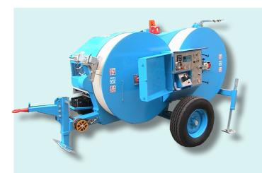
Hydraulic tensioner fit to string one conductor or fiber optic cable.
