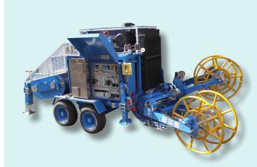
Hydraulic puller fit to pull one or two ropes in stringing operations of overhead transmission lines.
