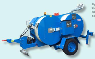
Hydraulic tensioner fit to string one or two conductors or optical fiber cables. One hydraulic circuit allows to tension at constant force even varying the speed of stringing.
