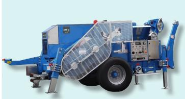
Hydraulic puller fit to pull one rope in stringing operations of overhead transmission lines.
