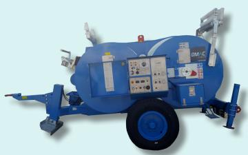
Hydraulic machine designed to operate both as a tensioner and as puller, fit to string 1, 2, 3 or 4 ropes or conductors.
